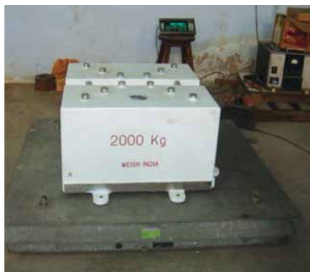
Fig.1.14 : Calibration set-up of 2000 kg weight of ISRO, Bangalore
