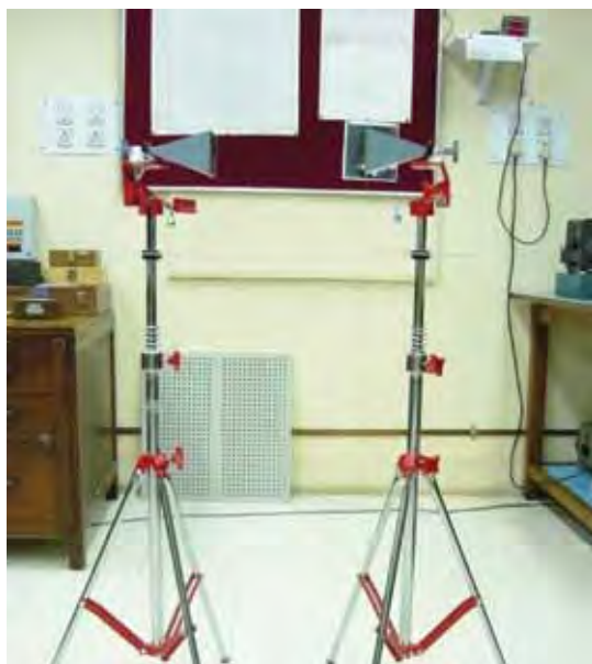
Fig.2.11 X-band horn antennas with turn tables
