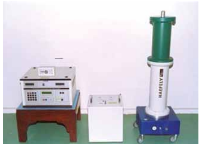
Fig. 2.7 The National Standard of AC High Voltage Ratio up to 100kV/100V comprising of the Compressed Gas Capacitor, Air Capacitor & the Electronic Voltage Divider (EVD)
