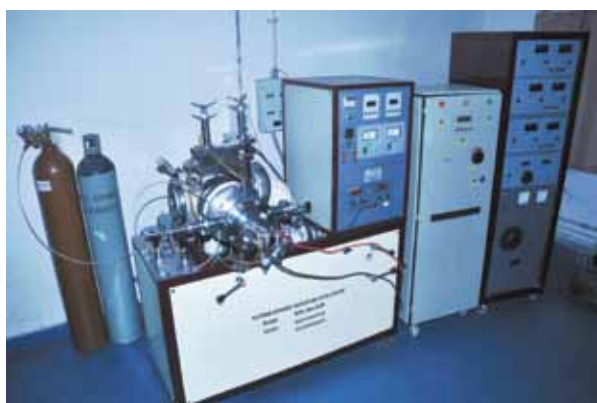
Fig. 4.10 Modified FCVA system integrated with CJCA and AJCA techniques
