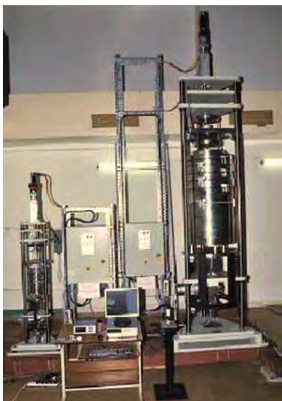
Fig.1.27 Brinell hardness primary standard machine
