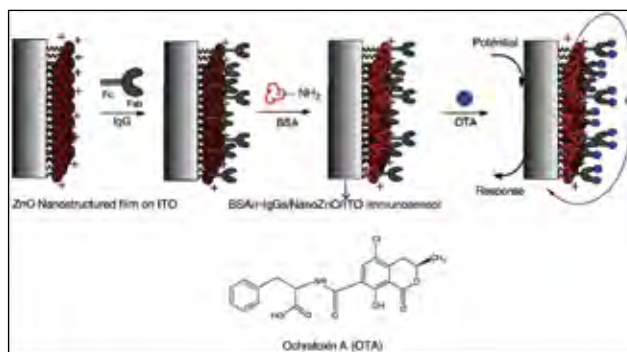
Fig. 3.24: Schematic of fabrication of BSA/r-IgGs/Nano-ZnO/ITO immunosensor along with the biochemical reaction between OTA and immunosensor.
