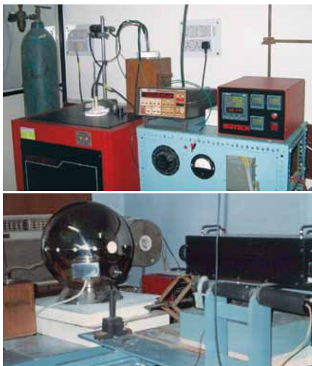
Fig.1.20 Set-up for Zn-point Calibration and Non-contact Comparison for Pt/Pd Thermocouple
