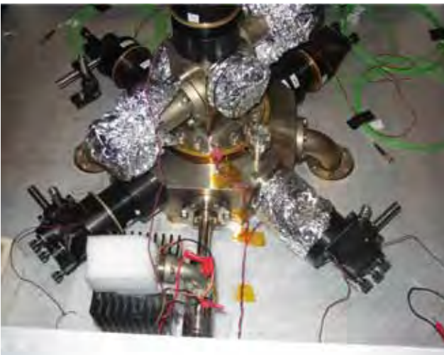
Fig. 2.2 MOT setup of Laser Cooled Cs Fountain Project
