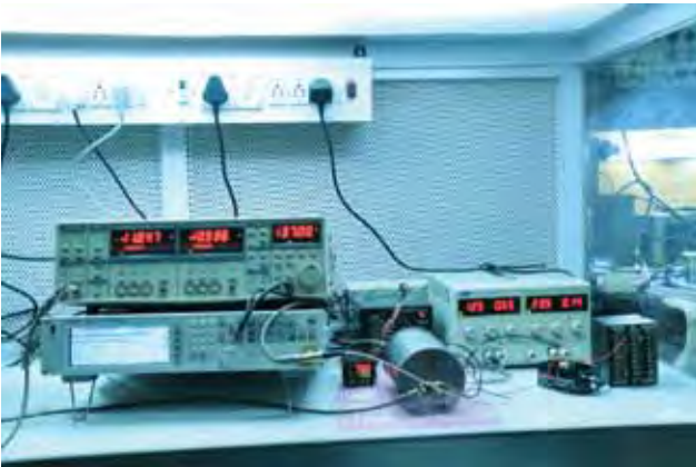
Fig. 2.1 Current Status of Physics package of Rb clock (SAC-NPL Project)
