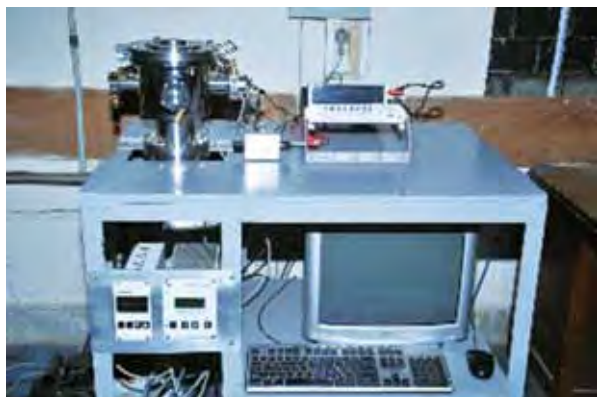
Fig. 4.11 Field emission measurement set up.
