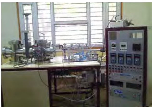
Fig 4.5 Microwave/VHF PECVD system for the deposition of amorphous and micro/nano crystalline silicon films
