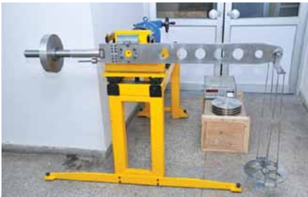
Fig.1.25. Torque primary standard machine developed for RRSL, Bangalore
