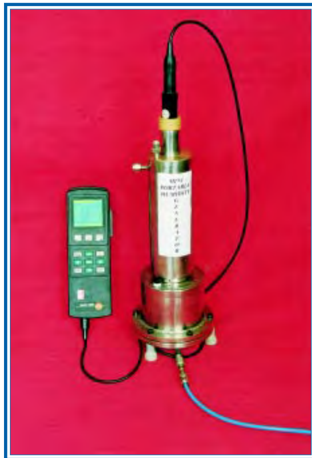
Fig. 7.3 : Simple and compact dew point generator (Mini RH generator)
