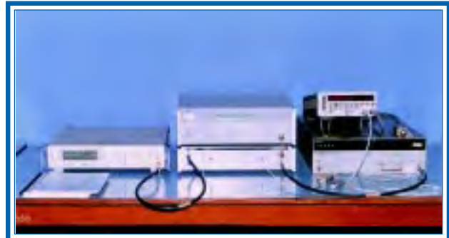
Fig. 2.5 Experimental set-up for the measurement of attenuation (18 – 40 GHz)
