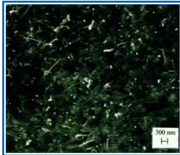
Fig.3.2 SEM photograph showing the dispersion of carbon nanotubes in the matrix pitch.
