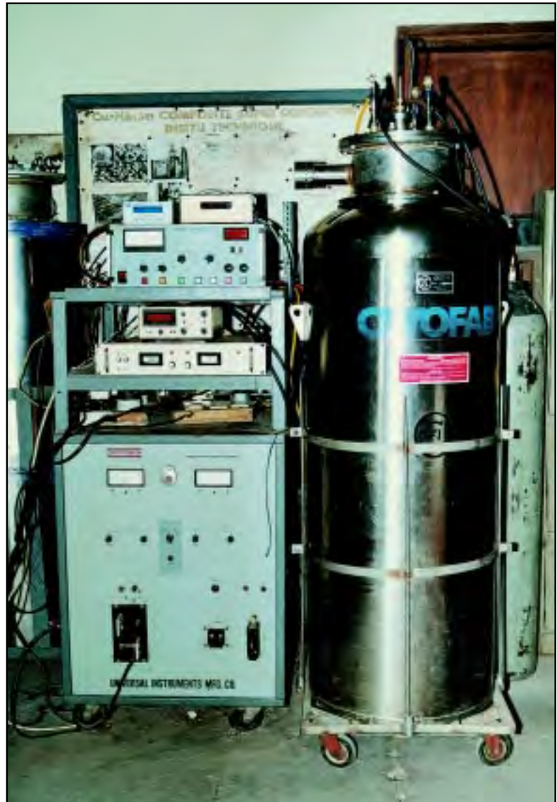
Fig. 7.6 : An 11 Tesla (50 mm bore dia.) SC magnet is being tested. The magnet with support system was mounted in the 10 inches bucket type dewar. The inner and outer coils were individually connected to the two power supplies 250A, 7.5 V and 100A, 5V respectively. Also seen in the photograph on the left side are Hall Effect Gaussmeter and liquid helium level meter
