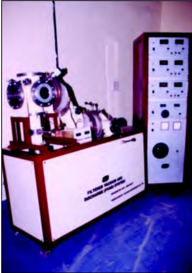
Fig. 4.5: Vacuum Plasma arc deposition system developed under a DST Project at NPL
