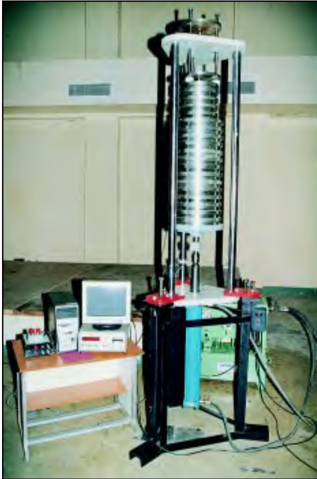
Fig. 1.9 : Dead weight force standard machine designed and developed at NPL
