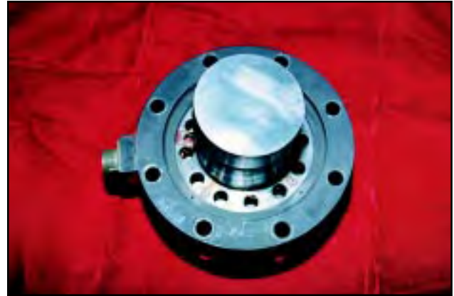
Fig. 1.10 : Multiple bending beam type force transducer designed and developed at NPL
