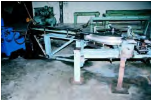
Fig. 3.1 : Hydraulically operated oval shaped tube bending machine with bent oval tube of Al alloy in annealed condition
