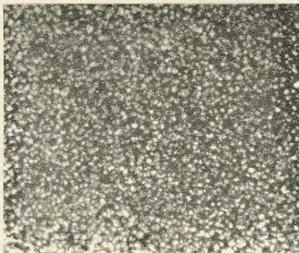
Fig. Optical micrograph of a polymer dispersed liquid crystal film under a polarizing microscope ( \times 400 magnification); LC droplets size \approx 5 \mu\text{m}
