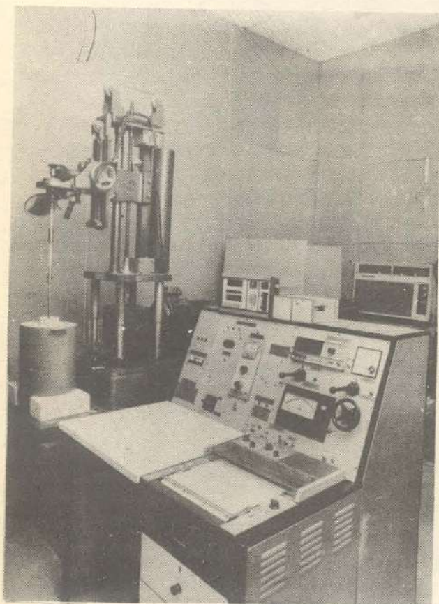
Fig.9. A versatile crystal puller designed, developed and fabricated at the NPL. It is being used for growth of nearly perfect single crystals from melt by the Czochralski method.
