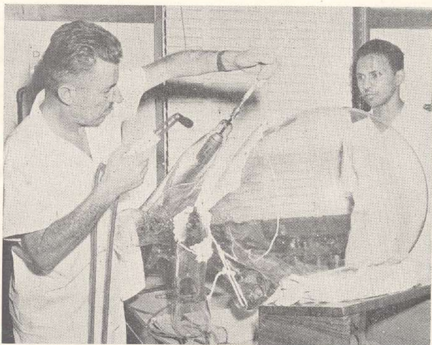
Fig. 5 Reconditioning of Mercury Arc Rectifiers being done at NPL.
