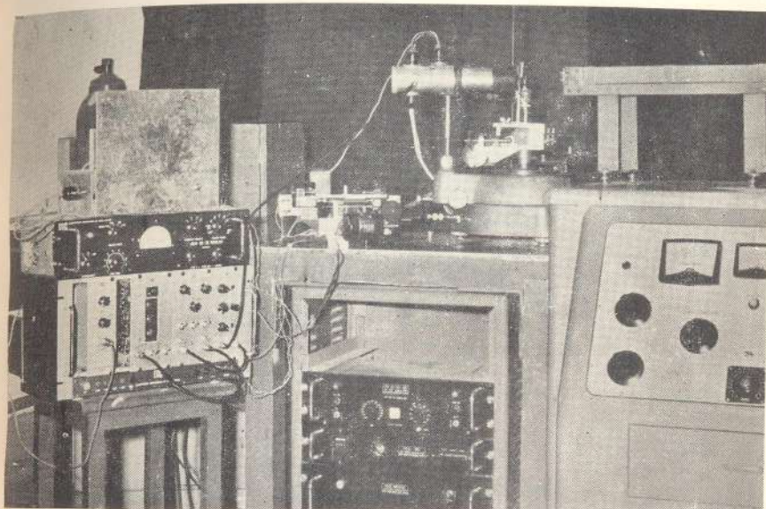
Fig. 2(a) The X-ray Diffraction Topography Camera designed and fabricated at NPL.
