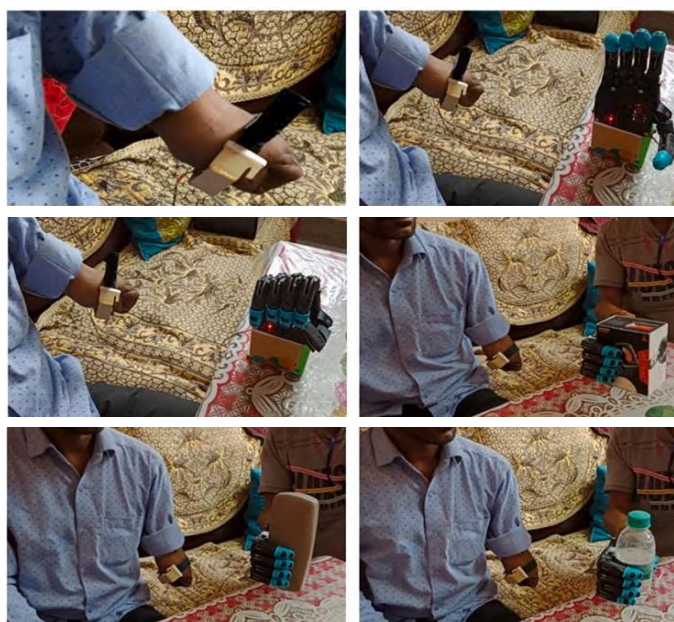
Trial of developed HMG sensor and 3D-printed hand on a transradial amputee
