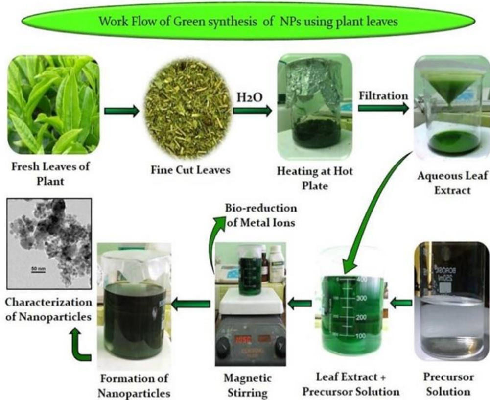
Workflow for green synthesis of nanoparticles using leaf extract
