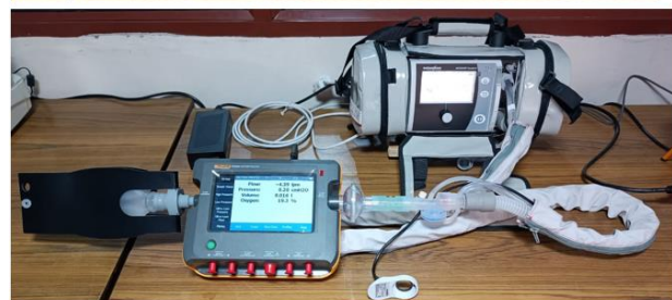
Set-up for calibration of ventilator using ventilator tester and electrical safety analyzer
