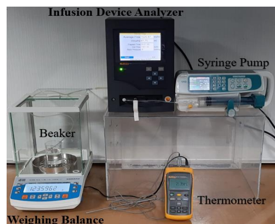
Low liquid flow calibration facility with main components: syringe pump, infusion device analyzer (IDA), beaker and weighing balance Standard 5 ml/hr to 1500 ml/hr
