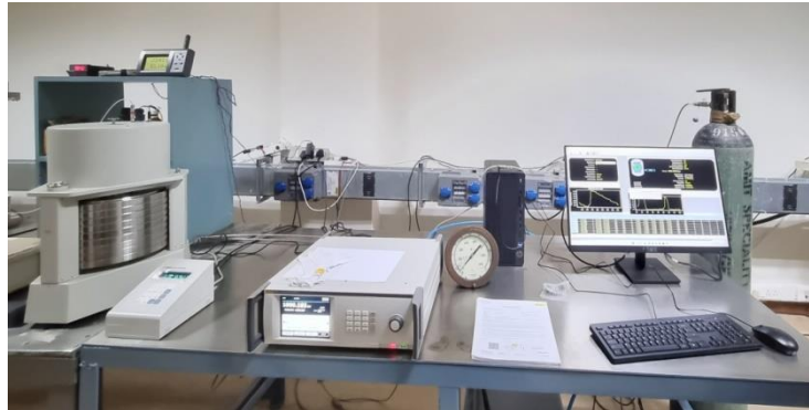
High pneumatic primary pressure standard from 0.2 MPa to 100 MPa
