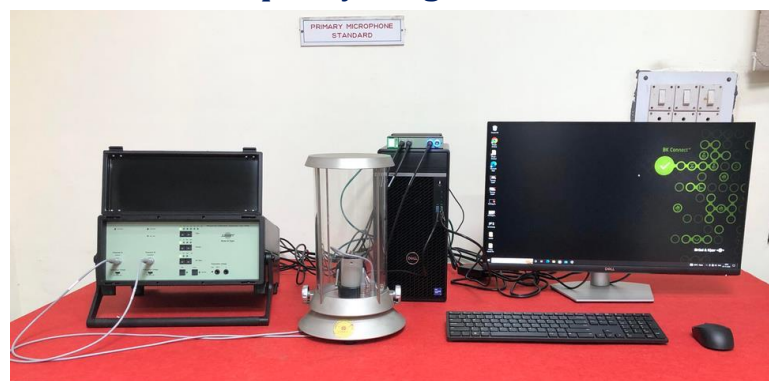
Upgraded primary sound calibration standard using reciprocity method in frequency range of 1 Hz to 25 kHz
