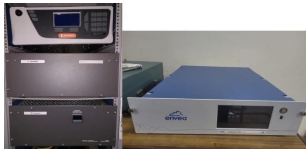
Secondary ozone standard for the calibration of ozone generators
