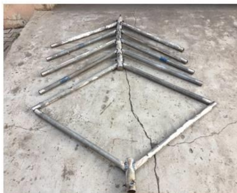
(e) Double Sided rod for Street Light
