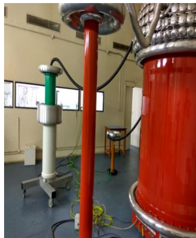
Calibration set-up for 200kV AC HV Divider
