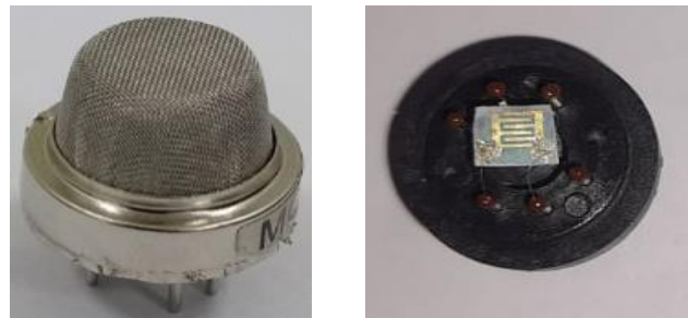
Portable NO 2 gas sensor based on In 2 O 3 thin film
