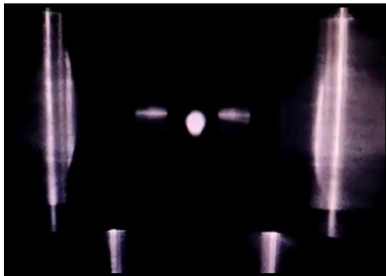
Image of laser-cooled cloud of Cesium atoms, trapped in a magento-optical trap (MOT), captured with an Infrared CCD camera mounted on one of the viewports on the vacuum chamber. In the bright spot (atomic cloud), more than 10 million Cesium atoms are trapped at few micro kelvin temperature. The cold Cesium atomic cloud is used to realize SI Second in India's first and only indigenously developed Cesium Fountain Primary Frequency Standard
