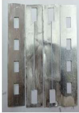
Fabrication of Aluminum Metal Mask
