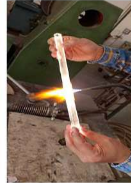
Vacuum sealing in quartz tube
