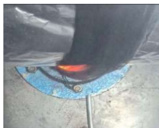
Winding of CNT sheet from FC-CVD
