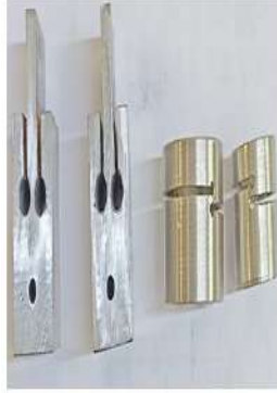
Fabrication of Hole Plates (Mild Steel)
